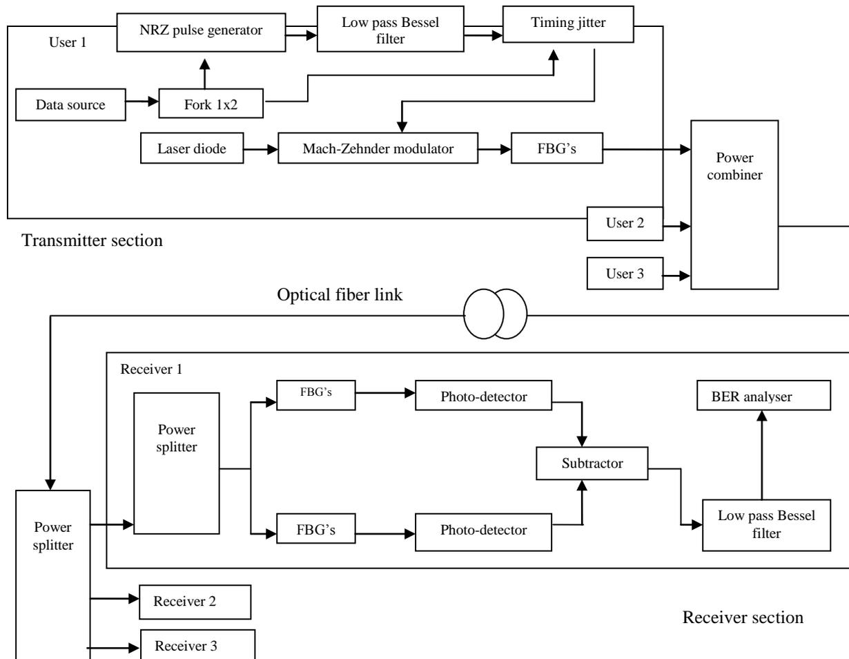
Fig 2: Block diagram for SAC-OCDMA system for 3 users.
