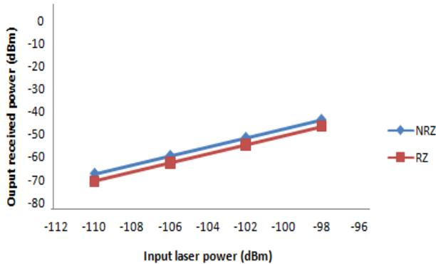
Fig 10: Received power Vs laser power for Corning TITAN fiber
