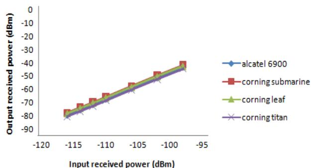
Fig 14: Received power Vs input laser for four fibers using NRZ data format
