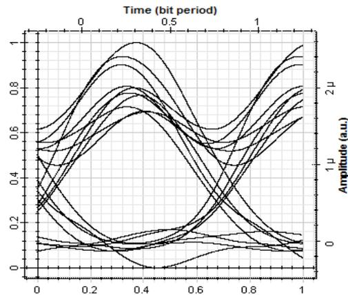
Fig 17: Eye diagram at -120 dBm input laser power for RZ format
