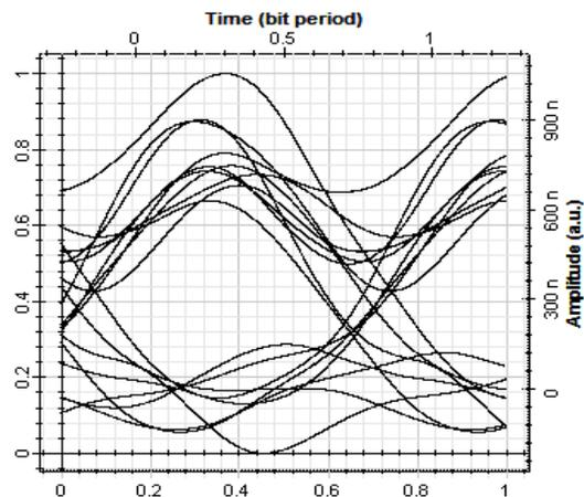
Fig 18: Eye diagram at -124 dBm input laser power for RZ format
