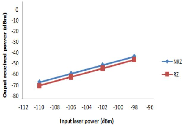
Fig 6: Received power Vs laser power for Corning Submarine fiber
