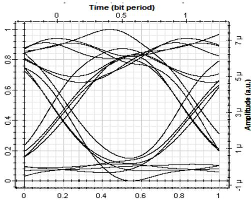
Fig 15: Eye diagram at -120 dBm input laser power for NRZ format
