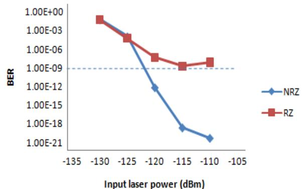
Fig 5: BER Vs input laser power for Corning Submarine fiber
