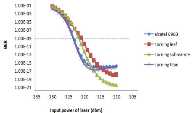
Fig 12: BER Vs input laser for four fibers using NRZ data format
