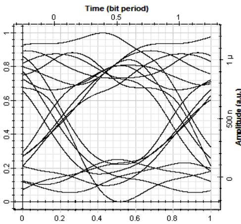
Fig 16: Eye diagram at -124 dBm input laser power for NRZ format
