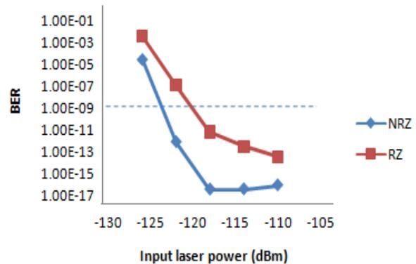
Fig 9: BER Vs input laser power for Corning TITAN fiber
