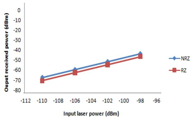
Fig 4: Received power Vs laser power for Alcatel 6900 fiber
