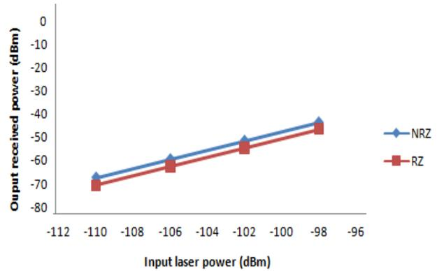
Fig 8: Received power Vs laser power for Corning LEAF fiber
