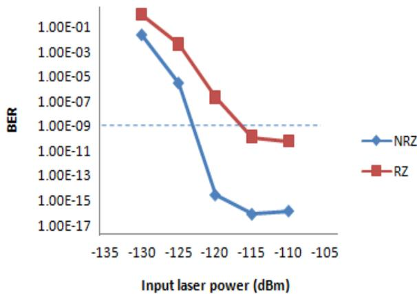
Fig 3: BER Vs input laser power for Alcatel 6900 fiber
