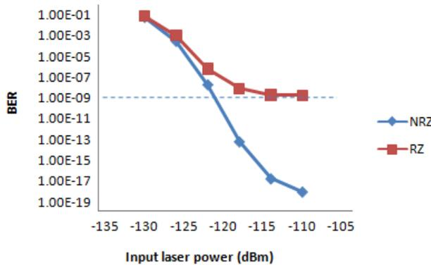
Fig 7: BER Vs input laser power for Corning LEAF fiber
