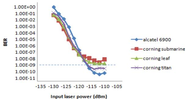
Fig 11: BER Vs input laser for four fibers using RZ data
