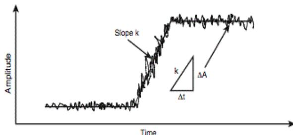
Fig 1: An ideal signal versus a noisy signal for a digital waveform
