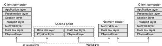
Fig 1: The OSI Protocol Stack and wireless communication
