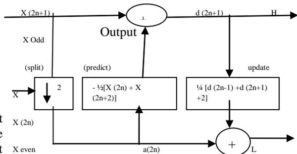
Figure 6. Lifting scheme decomposition of 5/3 filter
