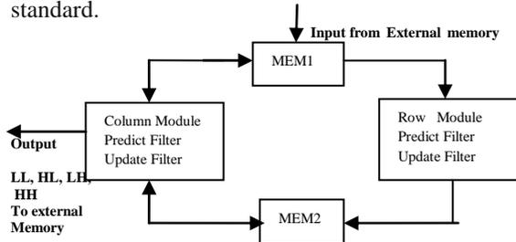
Figure 1. Lifting Based 2D DWT
