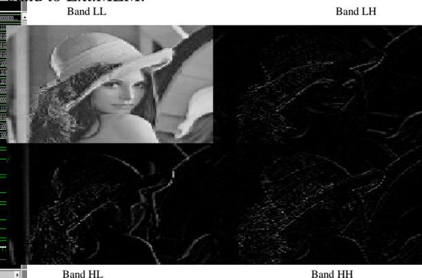
Figure 24. One level of 2D-DWT
