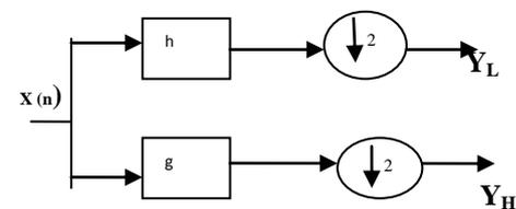
Figure 5. 1D DWT Decomposition
