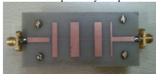
Figure 3. Photograph showing the Stepped Impedance low pass filter prototype without DGS
