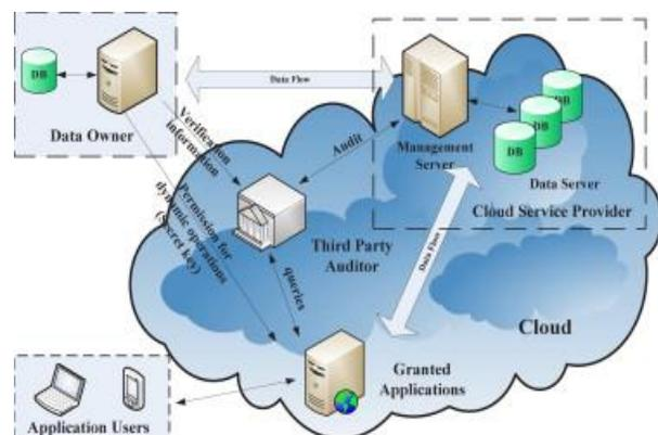
Fig 1: Cloud data storage architecture
