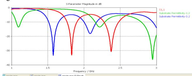
Figure 5 – Effect of substrate permittivity ( $\epsilon_r$ ) on antenna performance characteristics
