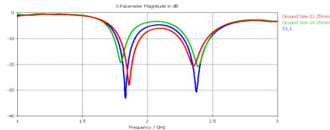
Figure 6: Effect of ground size variation on the antenna performance
