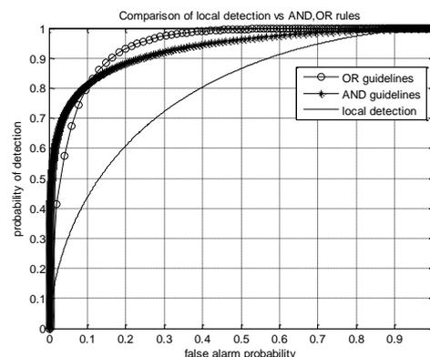
Fig 6 Comparison between OR,AND and local sensing
