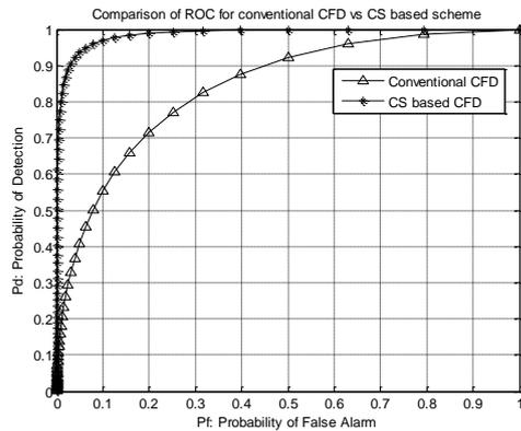
Fig 8 Comparison between CFD and CS-CFD
