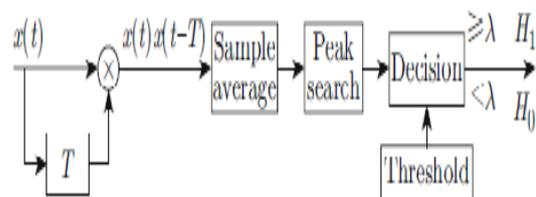
Fig 7 Cyclostationary Feature Detector
