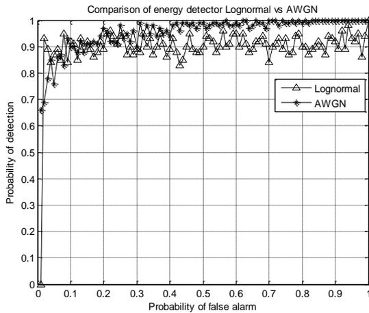
Fig 3 Energy Detection over AWGN and lognormal channels
