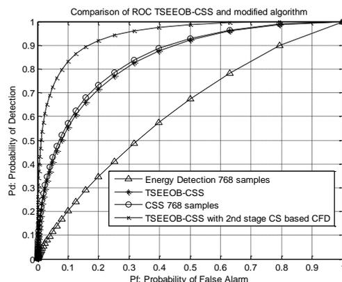
Fig 10 Comparison between ED, CSS, TSEEOB-CSS and modified algorithm
