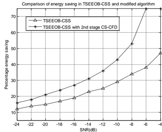
Fig 11 Energy Saving comparison TSEEOB-CSS vs modified algorithm
