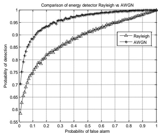
Fig 2 Energy detection over AWGN and Rayleigh channels
