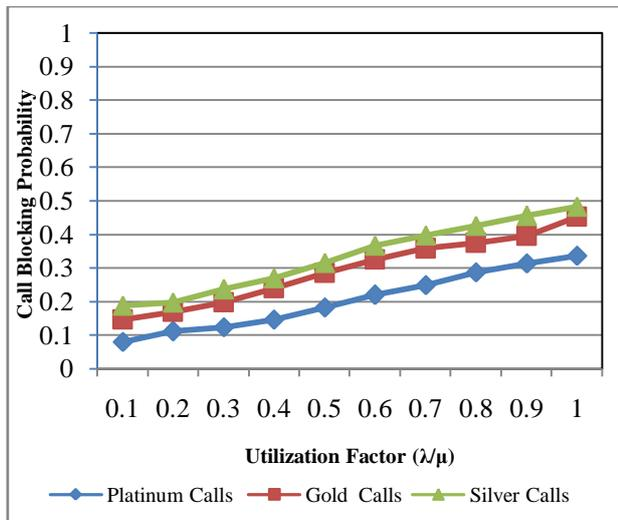
Figure 5: Call Blocking Probability of Different classes
