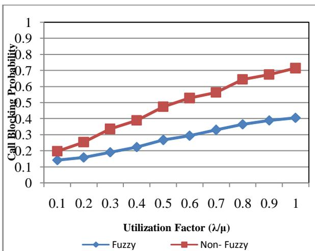
Figure 7: Call Blocking Probability with Fuzzy and Without Fuzzy comparison
