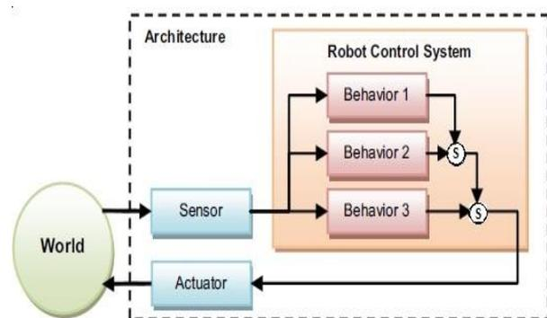
Fig 1: Subsumption based architecture
