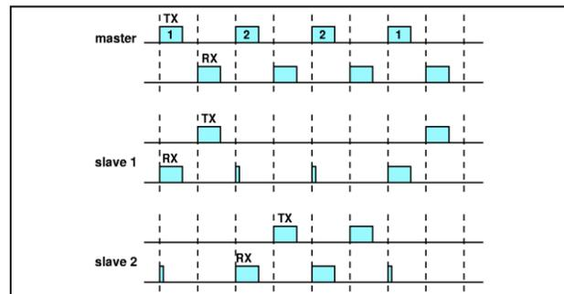
Fig. 6. Master/Slave transmits and receives timings
