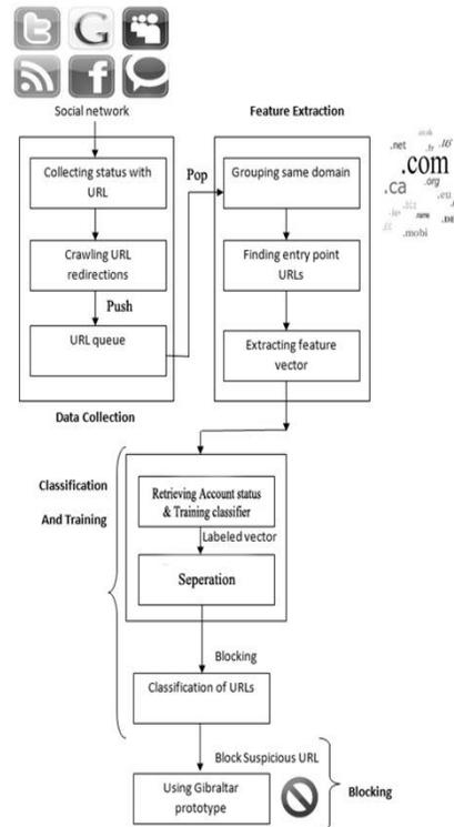
Fig. 2. System Architecture Design
