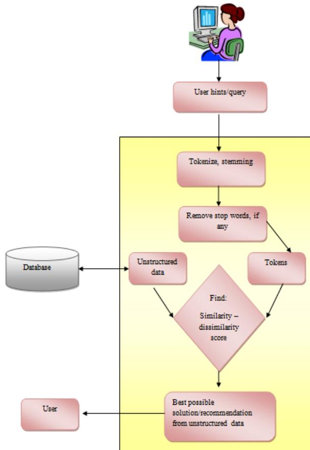
Fig. 2. Flow model of Algorithm-II for unstructured data
