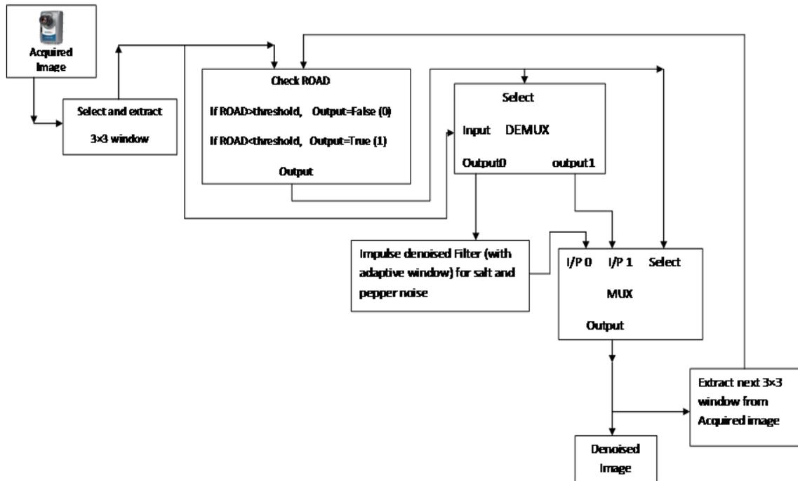
Fig.2: Architecture of Proposed Filter noise.
