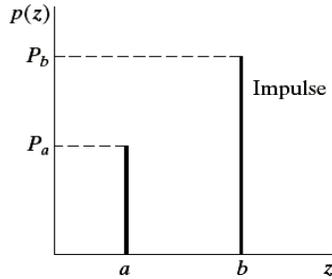
Fig. 1: Probability density function of impulse noise
