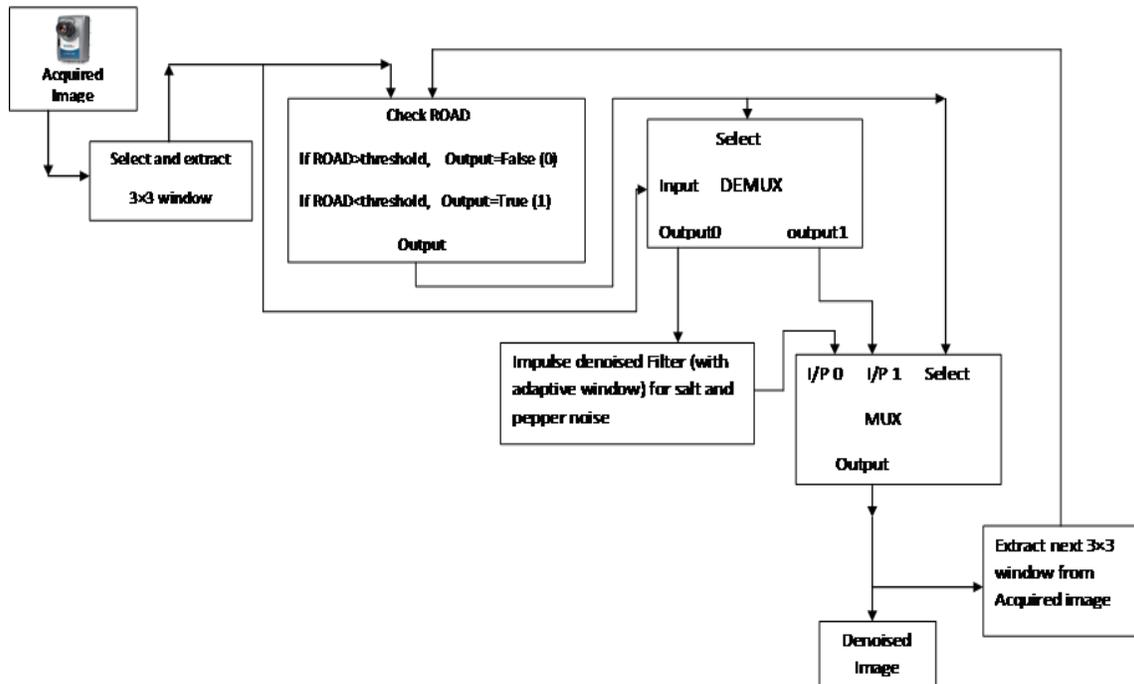
Fig.2: Architecture of Proposed Filter noise.
