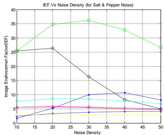
Fig.4: Performance comparison of various filters in terms of IEF, calculated on Test Image containing different noise levels of salt & pepper noise.
