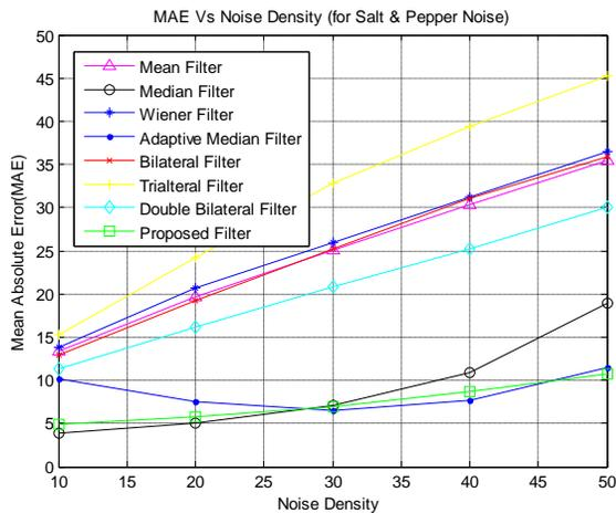
Fig. 3: Performance comparison of various filters in terms of MAE, calculated on Test Image containing different noise levels of salt & pepper
