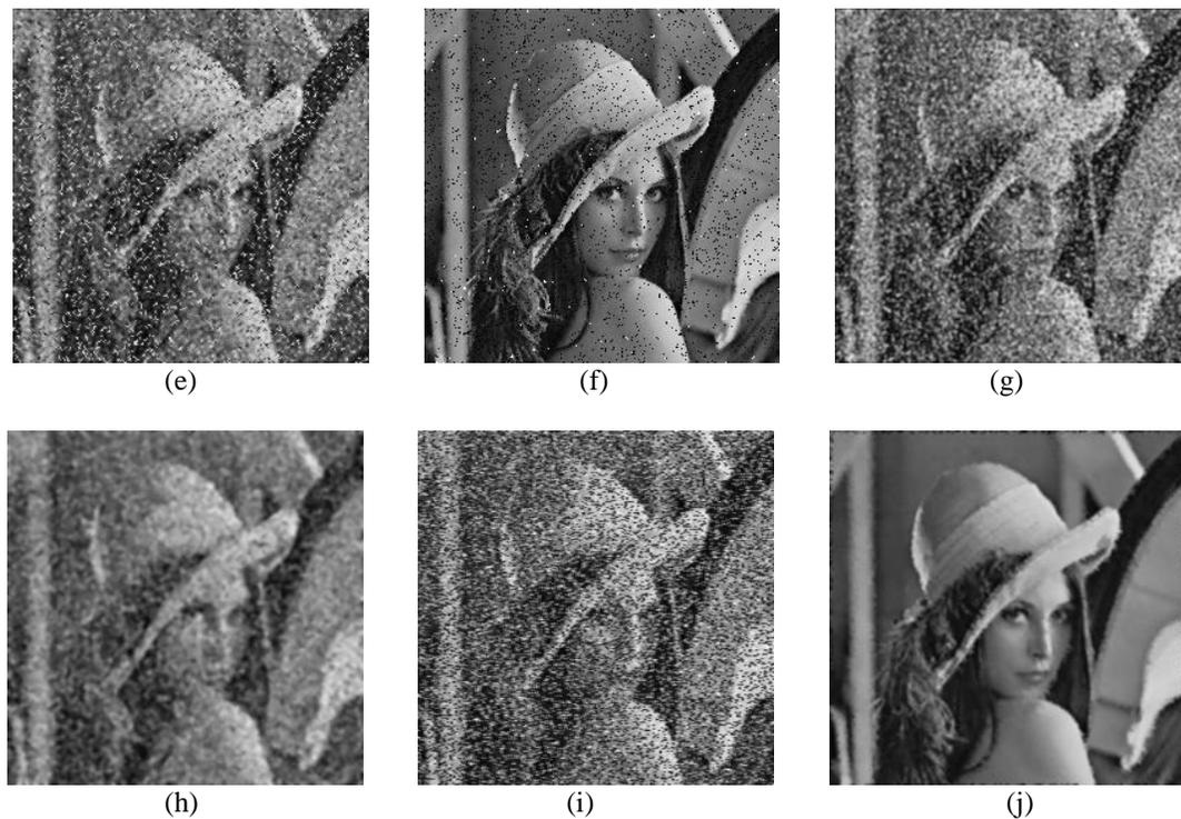
Fig.5: Performance of Various Filters for Lena Image corrupted with salt & pepper noise ( $\sigma_1$ (standard Deviation) = 30%) (a) Original image (b) Noisy image (c) –(j): Results of various filtering schemes (c) Output of Mean Filter (d) Output of Median Filter (e) Output of Wiener Filter (f) Output of Adaptive Median Filter (g) Output of Bilateral Filter (h) Output of Double Bilateral Filter (i) Output of Trilateral Filter (j) Output of Proposed Filter.
