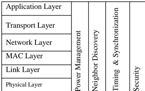
Fig 3. The protocol stack and cross-layer services.
