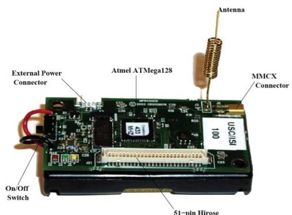
Fig. 2. A typical sensor node.
