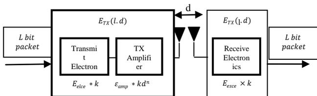
Fig.4. Radio energy dissipation model.
