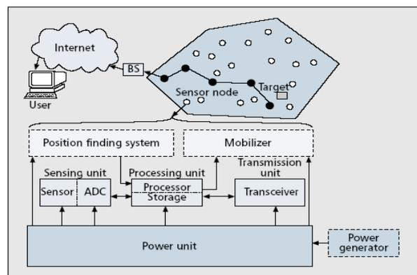
Fig. 1 Architecture of a sensor node.
