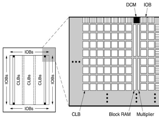
Fig 8: Internal structure of FPGA Configuration
