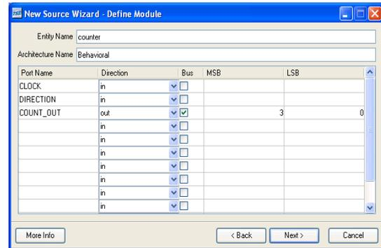
Fig 6: Declare the ports for the counter design by filling in the port information
