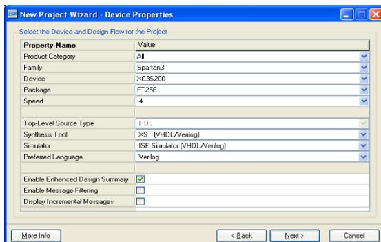
Fig 5: Creating a new ISE project for the FPGA device on the Spartan-3
