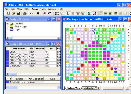
Fig 7: Pin locations for the ports
