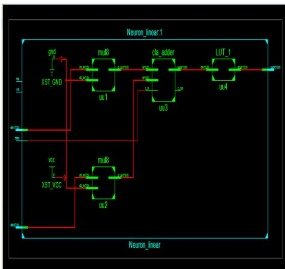
Fig 9. RTL schematic for single layer linear neuron
