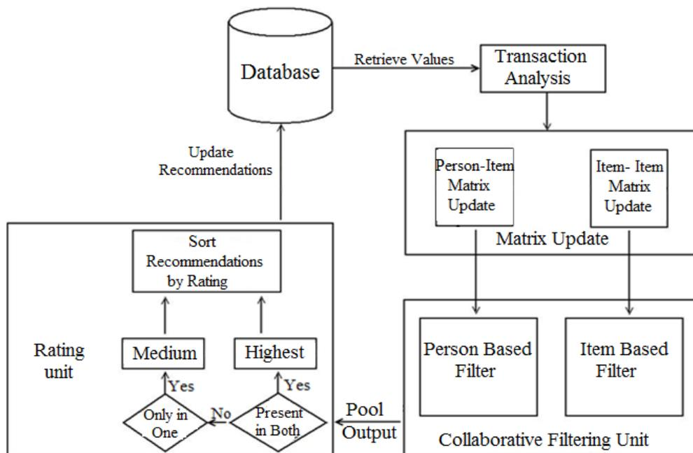
Fig.5. Block Diagram of Collaborative Filtering Tool
