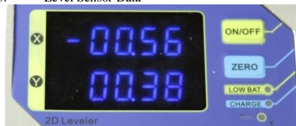
Fig.4 Level Sensor output which indicate X and Y axis tilt
