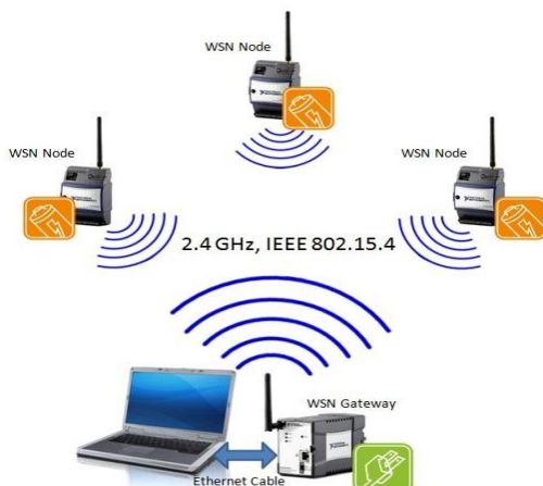
Fig. 1. Example of a wireless sensor network [9]
