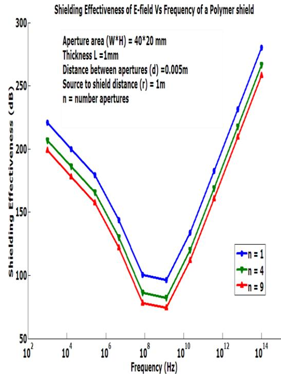
Fig 5.3: The variation of the Shielding effectiveness as a function of frequency for Polymer-E perforated shield with multiple apertures (n) for Electric field.
