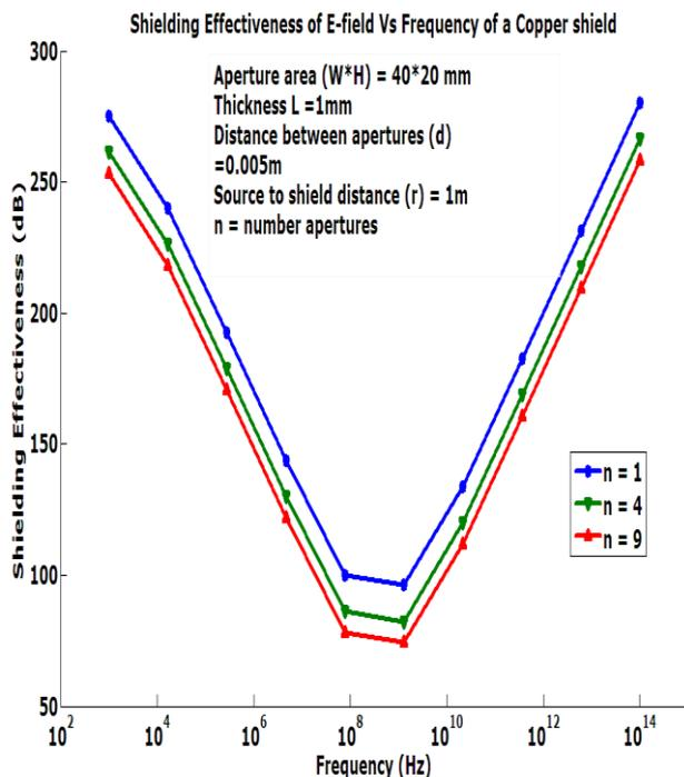
Fig 5.2: The variation of the Shielding effectiveness as a function of frequency for Copper perforated shield with multiple apertures(n) for Electric field.
