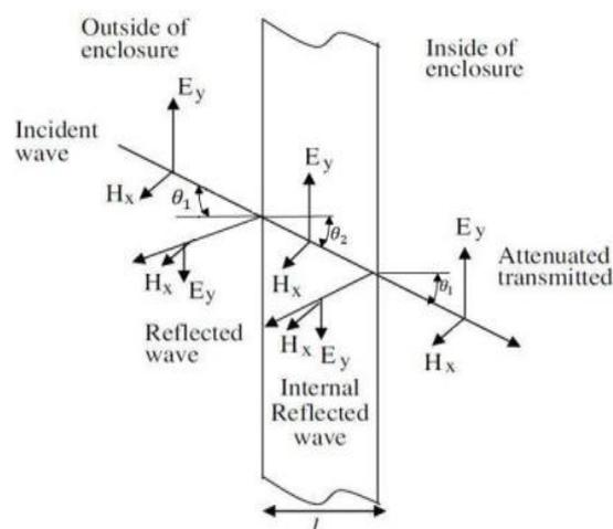
Fig. 1: Representation of shielding mechanisms for plane-waves
