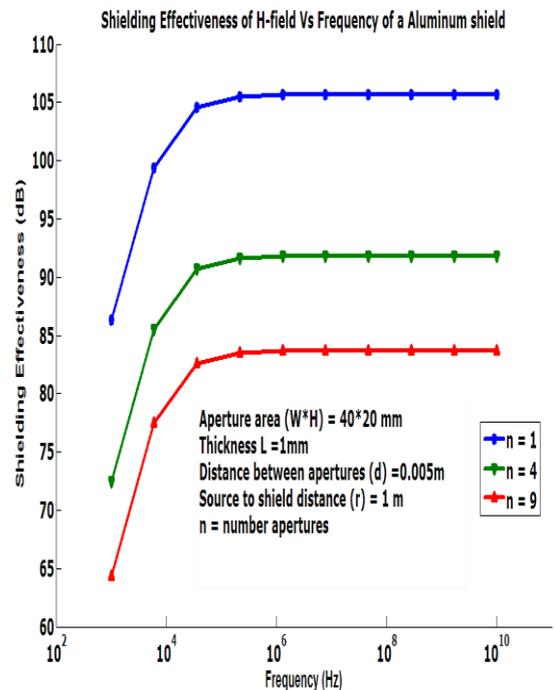
Fig 5.4: The variation of the Shielding effectiveness as a function of frequency for Aluminum perforated shield with multiple apertures (n) for Magnetic field.
