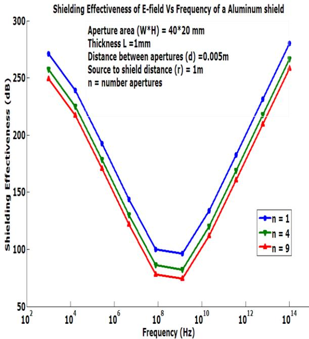
Fig 5.1: The variation of the Shielding effectiveness as a function of frequency for Aluminum perforated shield with multiple apertures (n) for Electric field.
