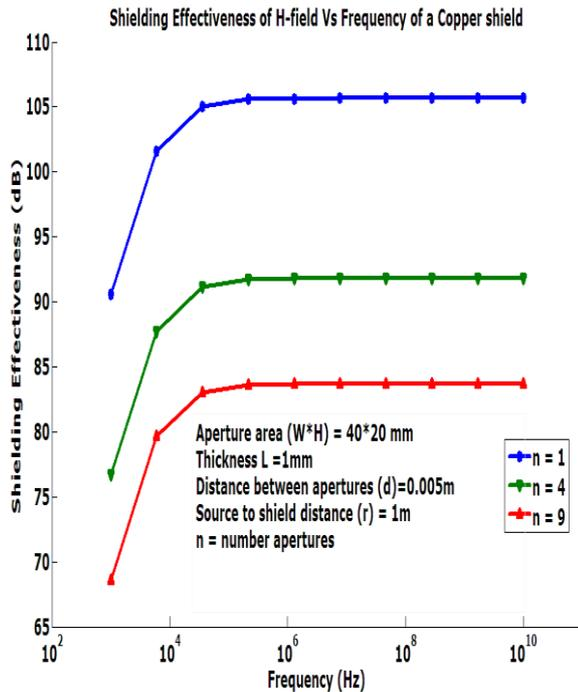
Fig 5.5: The variation of the Shielding effectiveness as a function of frequency for Copper perforated shield with multiple apertures (n) for Magnetic field.
