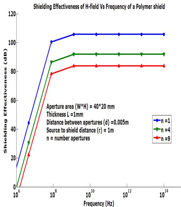
Fig 5.6: The variation of the Shielding effectiveness as a function of frequency for Polymer -E perforated shield with multiple apertures (n) for Magnetic field.
