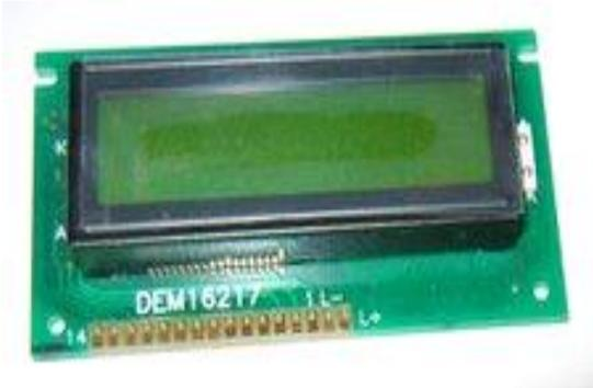
The HD 44780 is a liquid crystal dot matrix display Module that consists of LCD panel, LCD control driver, and driver and is capable of providing 16 characters x 2 lines display. It contains a controller, a data RAM and a character generator ROM required for providing display. Data interfacing is in 8-bit parallel or 4-bit parallel and data can be written in or read from a microprocessor.
