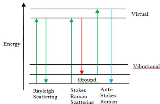
Fig. 2: Stokes and antiStokes process
