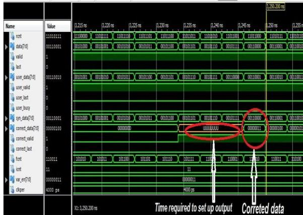
Fig.4 Simulation Waveform for RS (255,239) Decoder
