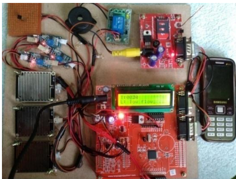
Fig 11: Output below 35% of water level
