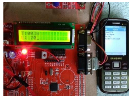
Fig 13: Output water level reaches 70%
