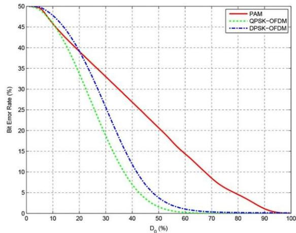
Fig.8. Effect of low pass filtering on BER performance. When cut off frequency is higher than 20%, OFDM based methods are superior to the PAM method.
