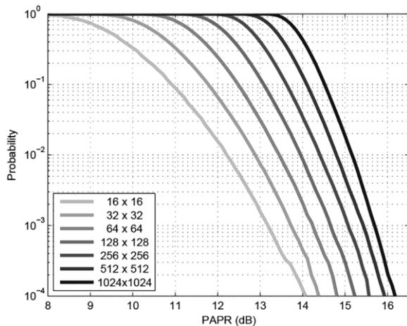
Fig.5. Probability that the OFDM modulated 2D signal has a PAPR greater than a certain value for different image sizes.
