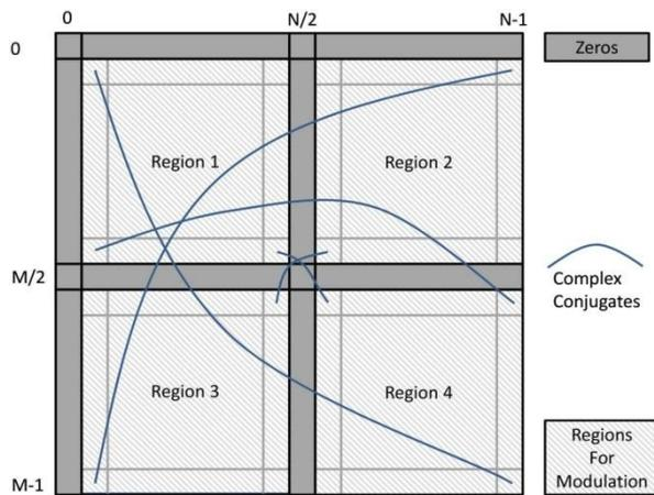
Fig.4. Hermitian symmetric matrix used for DPSK-OFDM modulation
