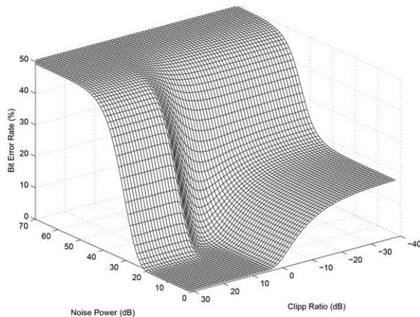
Fig7. Bit error rate vs. clip ratio and noise power. As noise level increases clip ratio should be increased in order to maintain optimum bit error rate.
