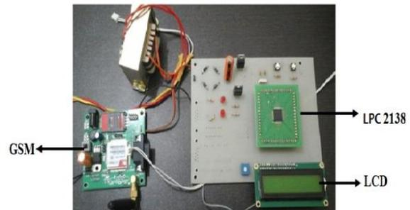
Fig.4. Hardware of server unit
