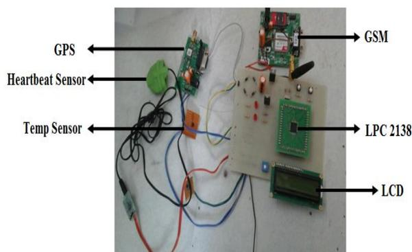
Fig.3. Hardware of mobile sensor unit
