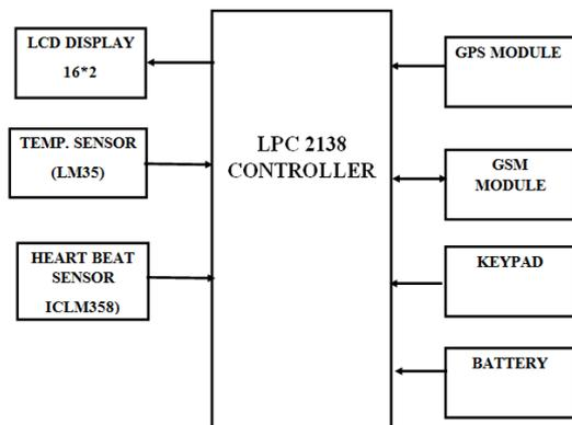
Fig.1. Block Diagram of Mobile Unit
