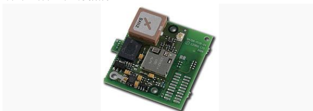
Fig2: Embedded serial-to-Wi-Fi module Increasingly in the last few years (particularly as of 2007), embedded Wi-Fi modules have become available that incorporate a real-time operating system and provide a simple means of wirelessly enabling any device which has and communicates via a serial port. This allows the design of simple monitoring devices.
