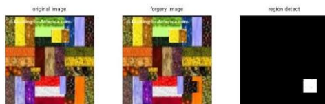
Figure 41 Illuminate image forgery example of 32X32
