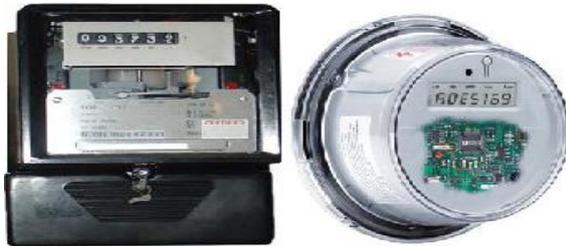
Fig.1 Traditional Electromechanical meter Vs Electronic meter.
