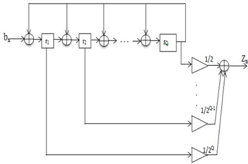
Fig 2: Inverse multi Tent map Finite state machine equivalent
