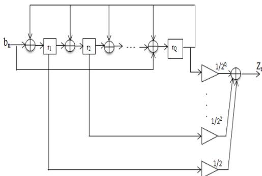
Fig 3: Multi Tent map Finite state machine equivalent
