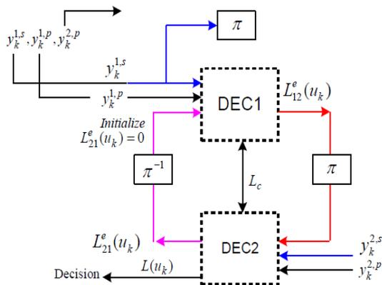
Fig 4: Iterative cycle of MAP decoding
