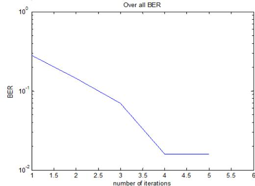
Fig 9: Plot of BER v/s number of iterations
