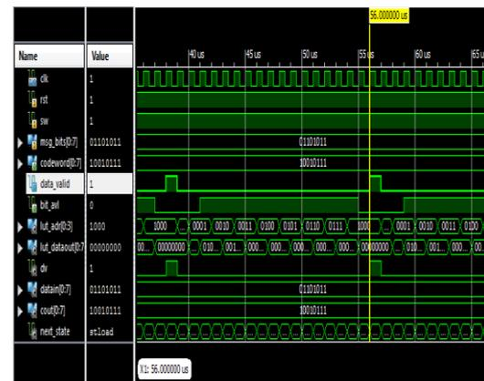
Fig 10: Output of chaos Turbo encoder
