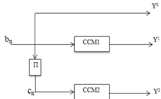
Fig 1: Chaos based Turbo encoder
