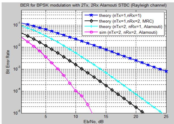
Fig7: BER for BPSK modulation for 2x2 Alamouti STBC
