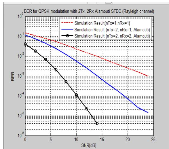
Fig8: BER for QPSK Modulation with 2x2 Alamouti STBC
