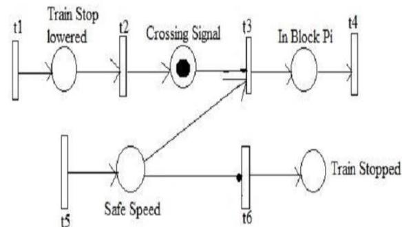
Petri net representation of Speed Checking in ATP
