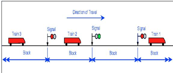
Figure 2: Diagram showing simple Metro-style two-aspect signaling.
