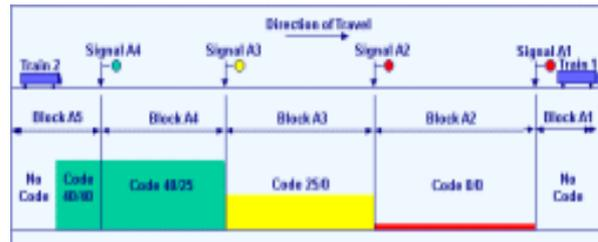
Figure 10: ATP Speed Codes
