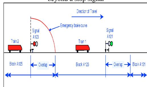
Figure 5: Diagram showing a signal provided with an overlap.
