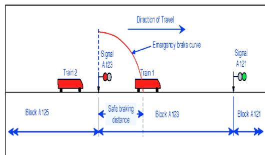
Figure 4: Diagram showing the need for a safe braking distance beyond a stop signal
