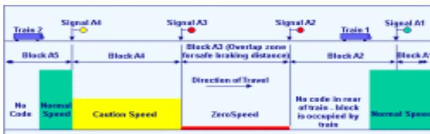
Figure 9: Electronic ATP
