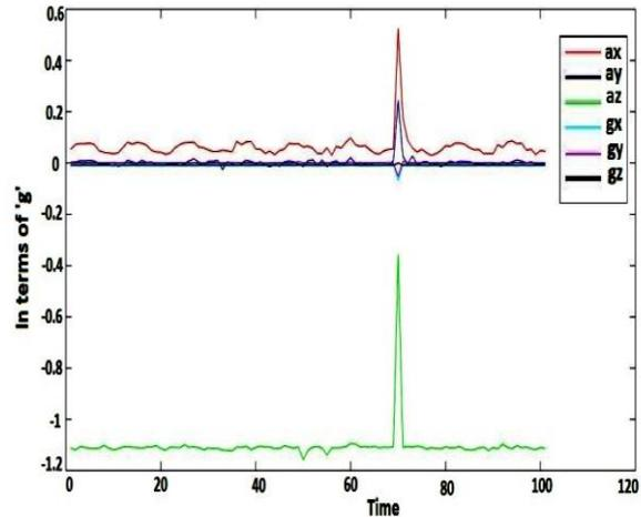
Fig.6.Hitting in X-direction
