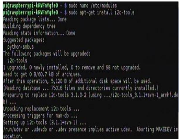
Fig.4. I2c tools installed
