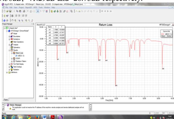
Fig. 3 Return loss of design antenna
