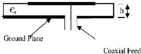
Fig. 1 Co-axial feeding technique
