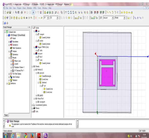
Fig. 2 Designed H-shape microstrip patch antenna
