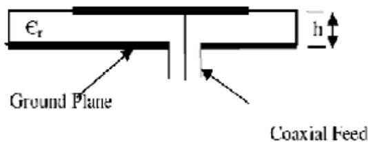
Fig. 1 Co-axial feeding technique
