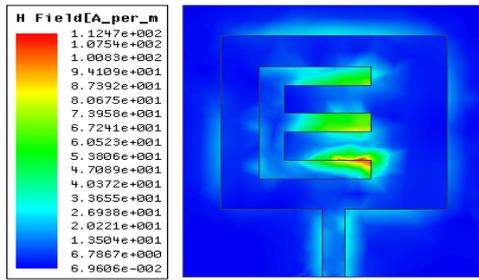
Fig.11.Simulated magnetic field distribution for the proposed antenna at 5.5 GHz
