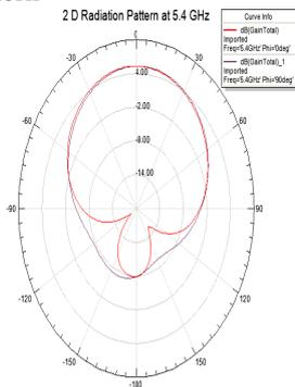
Fig. 12. Simulated 2-D radiation pattern at 5.4 GHz
