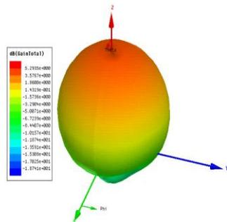
Fig. 13. Simulated 3-D radiation pattern of the E-slot patch antenna at 5.3 GHz
