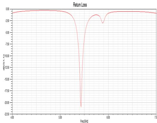
Fig. 6 Simulated plot of return loss
