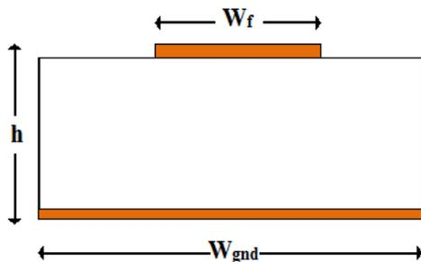
Fig. 3. Geometry of proposed microstrip-fed monopole antenna (Front View)
