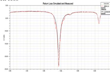
Fig.17. Diagram showing comparison between simulated and measured return loss
