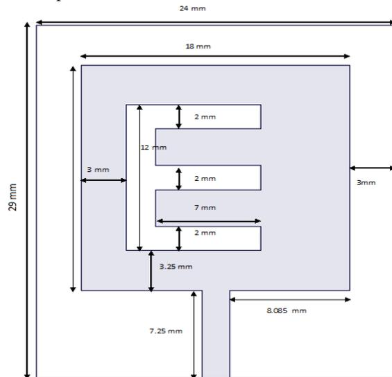
Fig.5 Dimensions of proposed E-slot patch antenna
