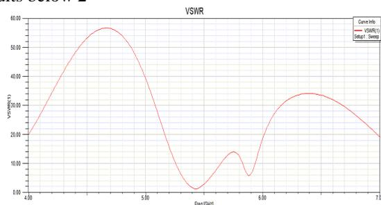
Fig.7. Simulated result of VSWR for proposed antenna
