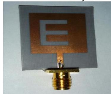
Fig.15. Front view of the fabricated prototype E-slot patch Antenna
