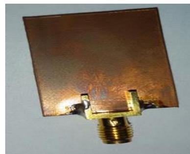
Fig.16. Back view of the fabricated prototype E-slot patch antenna
