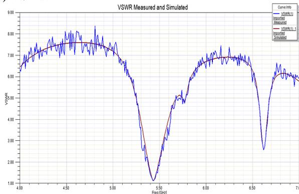
Fig. 18. Diagram showing comparison between simulated and measured VSWR
