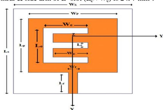
Fig. 1 Geometry of proposed microstrip-fed E-slot antenna (Front view)
