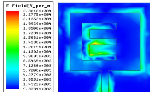
Fig.8. Simulated current distribution for the proposed E-slot patch antenna at 5.5 GHz
