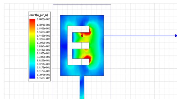
Fig.10. Simulated current density distribution for the proposed antenna at 5.4 GHz
