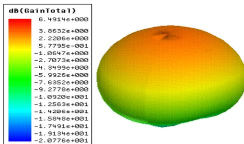
Fig. 14. Simulated 3-D radiation pattern of the E-slot patch antenna at 5.4 GHz
