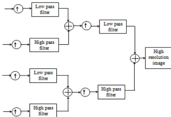
Fig 5: Block diagram of IDWT
