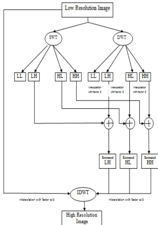
Fig 6: Flow chart for resolution enhancement
