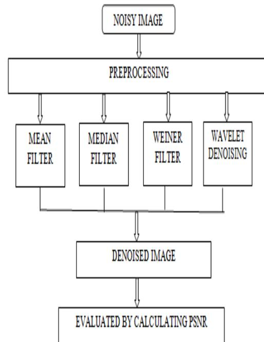
Fig 1: Flowchart for denoising technique
