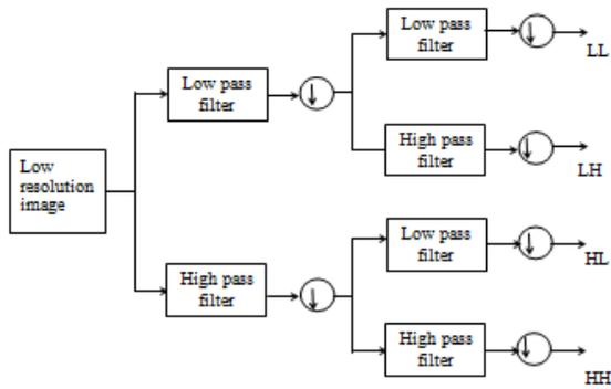
Fig 3: 2D DWT block diagram
