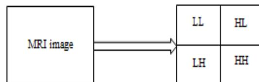
Fig 2: One level decomposition of DWT
