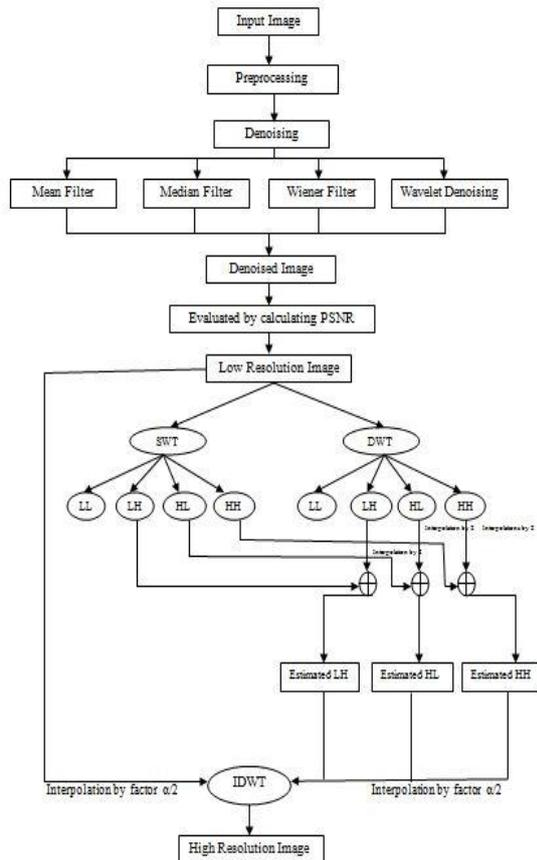
Fig 7: Final flow chart of proposed method
