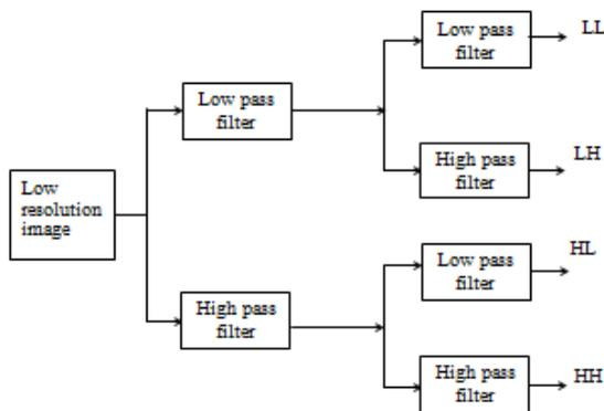
Fig 4: Block diagram of SWT
