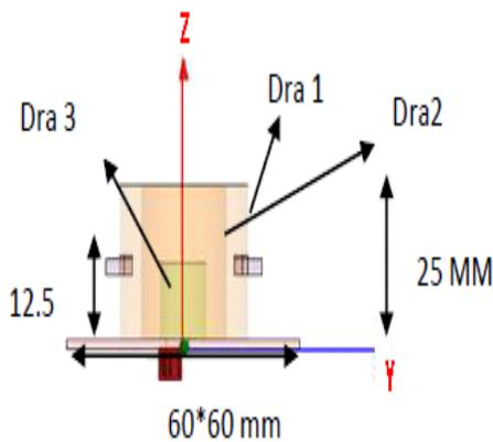
Fig. 2: Proposed Hybrid MHD Antenna (Side View)
