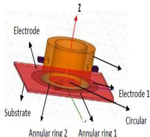
Fig. 1: Proposed Hybrid MHD Antenna (Front View)
