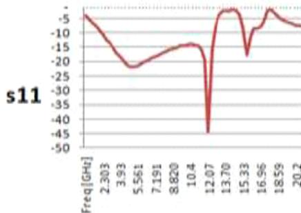
Fig. 3: Return loss without using stacked DRA
