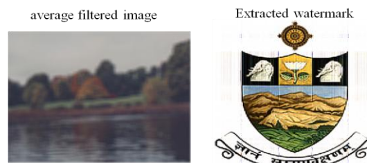
Fig. 9 Effect of Average filtering on watermarked image and extracted watermark
