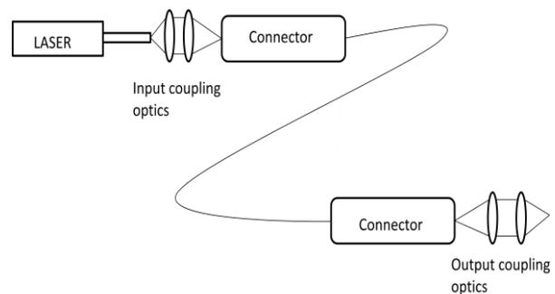
Fig.1. Fiber optic beam delivery system.
