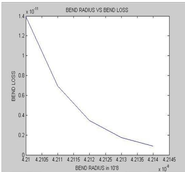
Fig .7.Theoretical bending loss as a funtion of bend radius. HCS fiber with core diameter of 198  $\mu\text{m}$  and  $\text{NA}=0.37$ .
