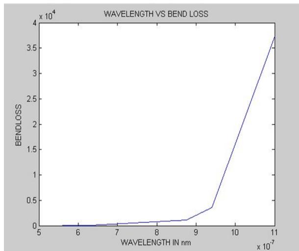
Fig.5. Theoretical bending loss as a function of Wavelength. HCS fiber with NA=0.37.
