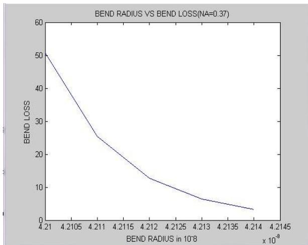
Fig.3. Theoretical bending loss as a function of bend radius. HCS fiber with NA=0.37.
