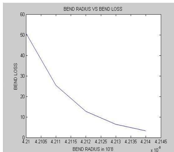
Fig.6. Theoretical bending loss as a function of bend radius. HCS fiber with core diameter of 200 μm and NA=0.37.
