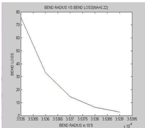
Fig.4. Theoretical bending loss as a function of bend radius. All-Silica fiber with NA=0.22.
