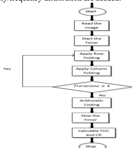
Fig: Flow Chart for Compression Procedure
