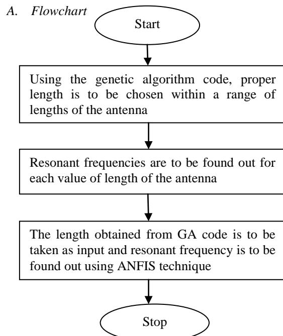
Fig. 2.3. Flowchart for GA-ANFIS hybrid technique.
