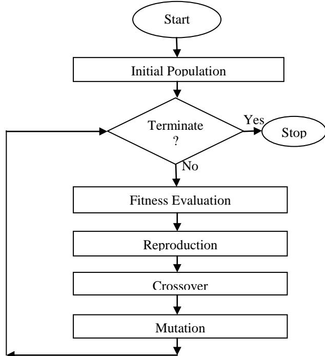
Fig. 2.1.Flowchart for Genetic Algorithm.
