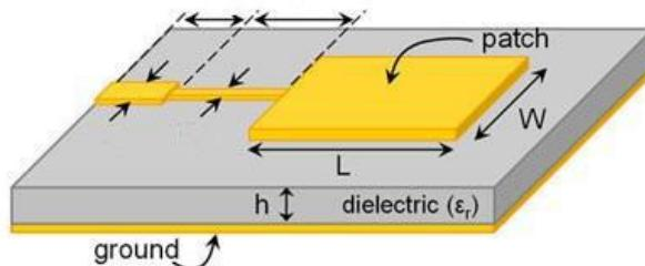
Fig. 1.2.Structure of a patch antenna.
