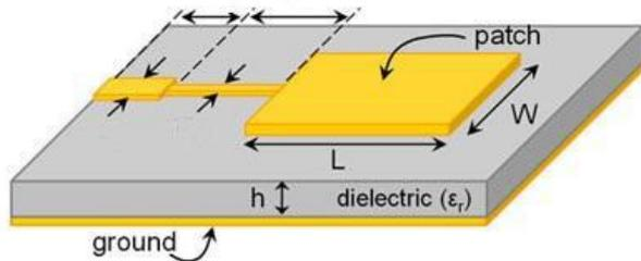
Fig. 1.2. Structure of a patch antenna.
