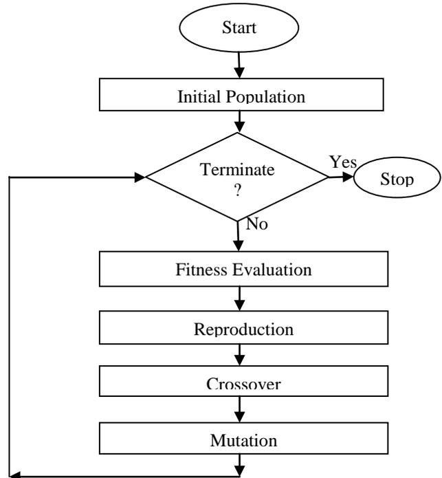
Fig. 2.1.Flowchart for Genetic Algorithm.
