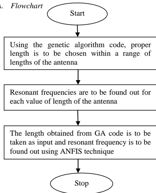
Fig. 2.3. Flowchart for GA-ANFIS hybrid technique.
