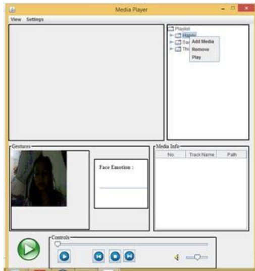
Fig 1: In this snapshot, the list of options are given to the user to maintain his/her song collection. The user can perform add Media operation, or remove the added media and can manually play the song.
