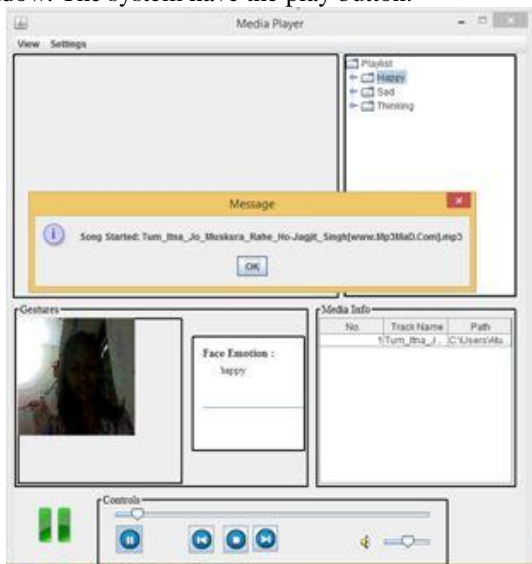
Fig 3. In the above snapshot, the emotion detection is started by pressing the play button. And the system has detected the emotion as "Happy". And the emotion-specific-playlist is created.
