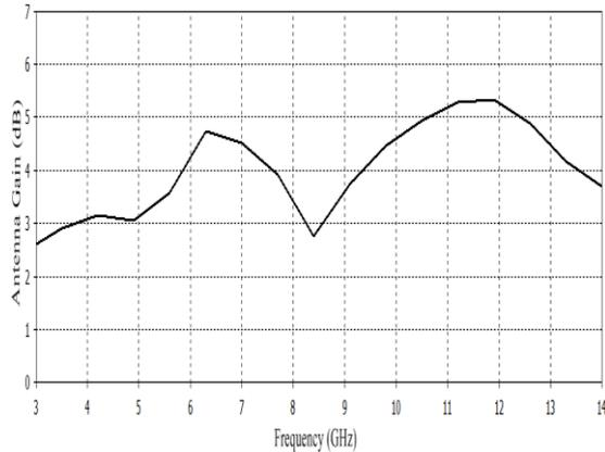
Fig. 7. Gain of the antenna.
