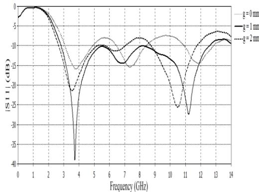
Fig. 2. Simulated return loss curves for  $g = 0$  mm,  $g = 1$  mm and  $g = 2$  mm.
