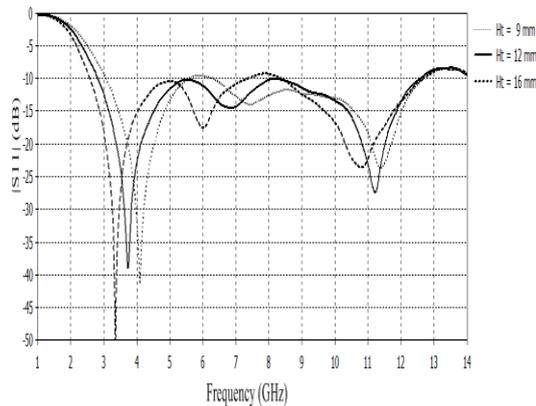
Fig. 3. Simulated return loss curves for  $H_t = 9$  mm,  $H_t = 12$  mm and  $H_t = 16$  mm.
