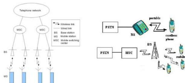
Fig.1: Basic mobile communication structure
