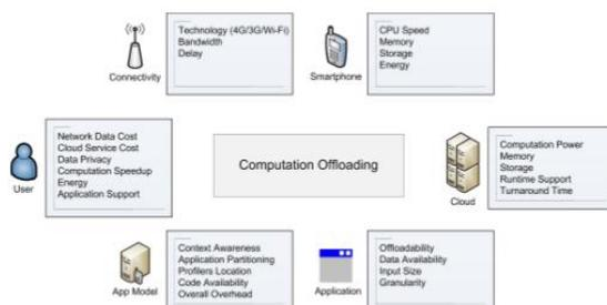
Fig. 3: Entities affecting computation offloading
