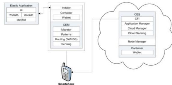
Fig. 5: Architecture of Zhang et al. Model
