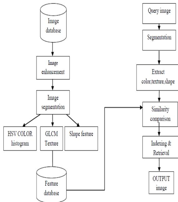
Fig.1 Block diagram of CBIR using combination of color, texture, shape.
