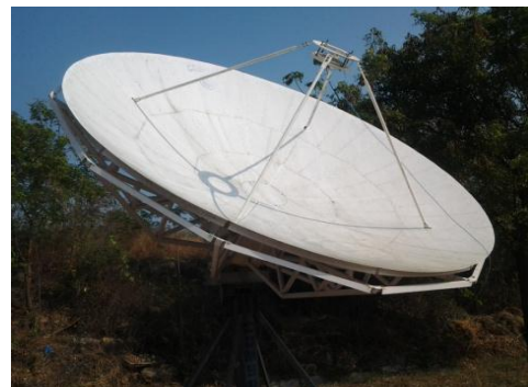
Fig 17: Parabolic Reflector Dish at NARL
