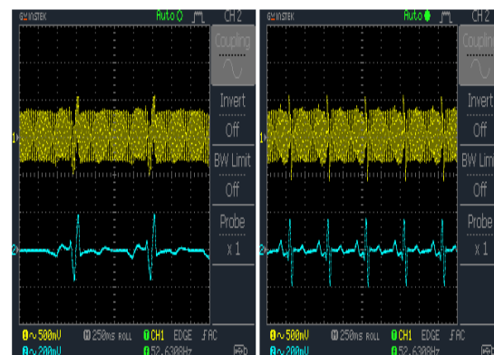
Fig. 9: Input and output signal of the digital LPF without interference signal
