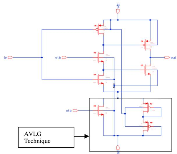
Figure 2.2 D Flip-flop designed using AVLG technique
