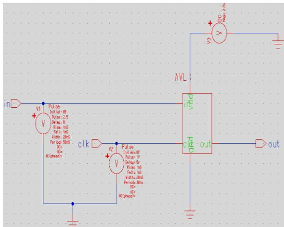
Figure 2.3 Test circuit of D Flip-flop Using AVLG Technique
