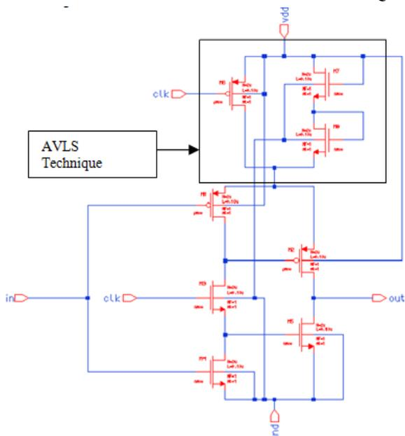
Figure 3.1 D Flip-flop designed using AVLS technique
