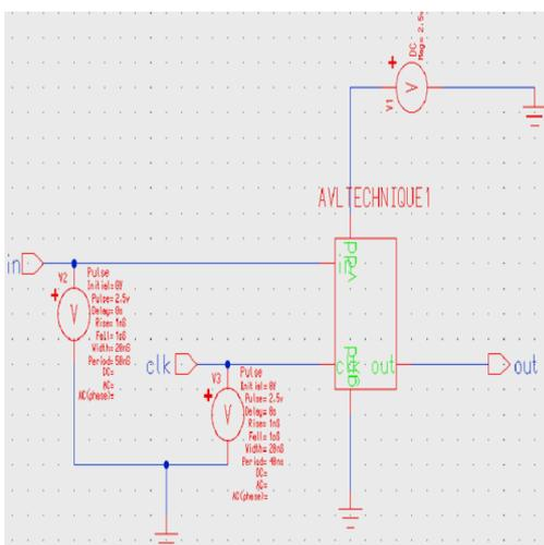
Figure 3.2 Test circuit of D-Flip flop Using AVLS Technique
