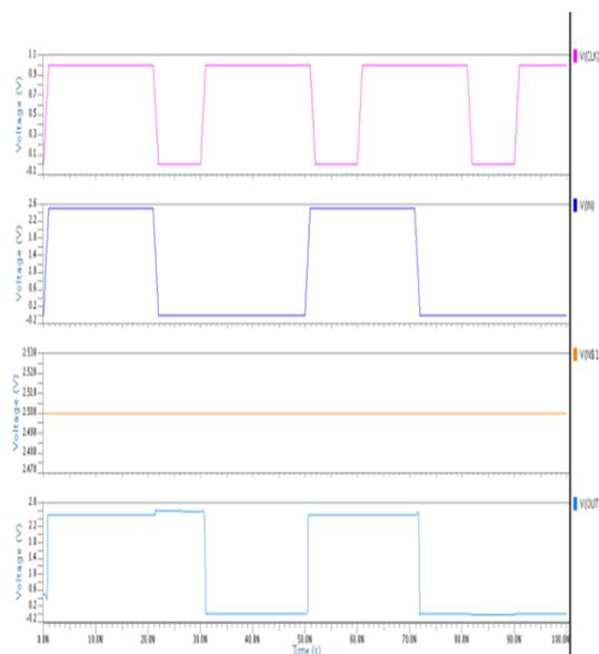
Figure 4.2 Simulation of D Flip-flop designed using AVLS technique
