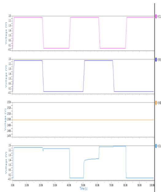
Figure 4.1 Simulation of D Flip-flop designed using AVLG technique
