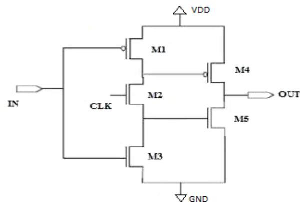
Figure 2.1 Basic TSPC based D Flip-flop
