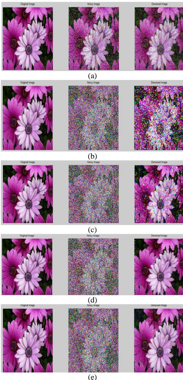
Fig 6.Results of different algorithms for color image.(a) Output of mean filter (b) Output of MF. (c) Output of AMF. (d) Output of DBAMF.(e)Output of MDBUTMF. for 70% noise density respectively.
