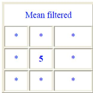
Fig 3: In this Centre value which is previously 1 in the unfiltered value is replaced by the mean of all nine values that is 5.
