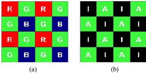
Fig. 1 . (a) The Bayer's filter mosaic; (b) The lattice A for the acquired green channels and the complementary lattice B for the interpolated green channels.
